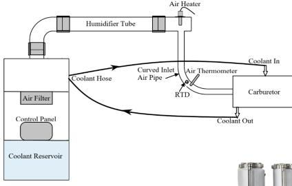
**The Cooling Circulation System** circulates coolant to the carburetor of the octane engine and to the fuel bowl that needs to be cooled by means of a specialized pump, through coolant hoses with quick couplings.
