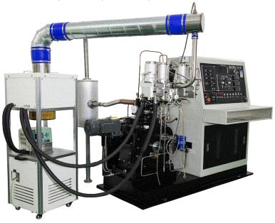
The intake air control system is installed in a movable industrial cabinet, suitable for different laboratory space conditions.
