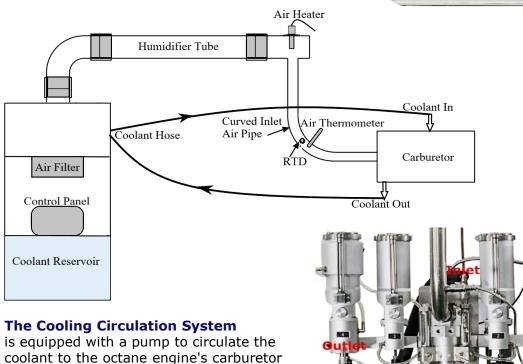
Plastic hoses are used for connecting to the carburetor by the quick couplings for cooling the carburetor.
