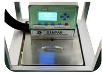
**The refrigeration system** is equipped with a separate stainless-steel reservoir of 10-liter refrigerating liquid. The temperature range of the cooling fluid could to be from ambient temperature to -10°C with the stability of 0.5°C. The refrigerating temperature and refrigerating time are adjustable, using a digital control panel.
